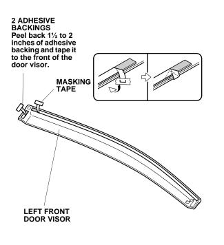
6. Position the left front door visor onto the left front door by inserting bracket B between the door mirror base and glass run channel as shown.
