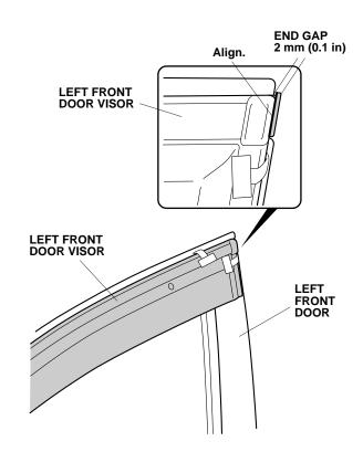
9. While applying light pressure against the left front door visor, carefully remove the adhesive backings in the order shown. Use your finger to push up each bracket so there is no gap between the bracket and the door sash.
