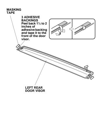
16. Align the clip holes in the left rear door visor with the bracket holes, and install the clips while pushing up on each bracket A. There should be no clearance between the brackets and the door sash. NOTE: Be sure the bracket and the door visor are aligned properly. Once the clip is installed, it cannot be reused.
