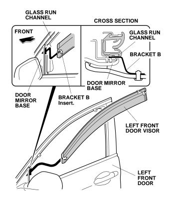
7. Align the clip holes in the left front door visor with the bracket holes, and install the clips while pushing up on each bracket A. There should be no clearance between the brackets and the door sash. NOTE: Be sure the bracket and the door visor are aligned properly. Once the clip is installed, it cannot be reused.
