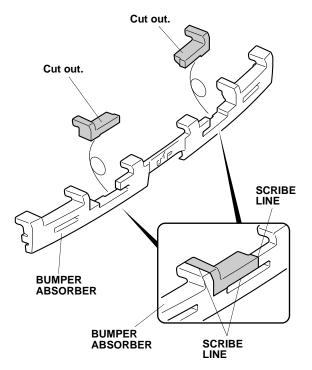
80. Reinstall the bumper absorber to the rear bumper beam.
