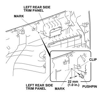
58. While wearing eye protection, drill the pierced mark with a 3 mm drill bit. Enlarge the hole with a 26 mm hole saw. Remove any burrs.
