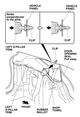
19. Using a rubber mallet wrapped with a shop towel, lightly tap the area marked "SIDE CURTAIN AIRBAG" on the left D-pillar trim to push in the clip. Make sure to tap perpendicular to the pillar. 20. Remove the left D-pillar trim (ten clips).
