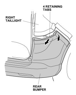
• With the help of an assistant, remove the rear bumper. Place the rear bumper on a blanket.
