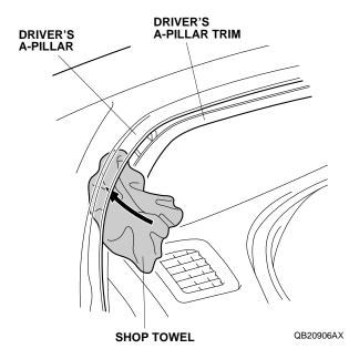
12. Slide the driver's A-pillar trim up to remove it from the upper clip. Carefully remove the shop towel and any clips that fell from the driver's A-pillar trim.
