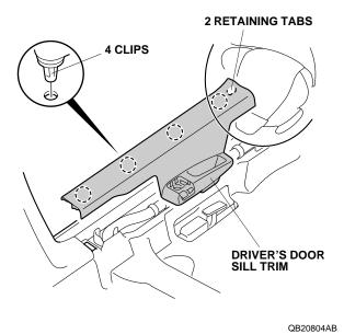
2-Door: Two retaining tabs and six clips.
