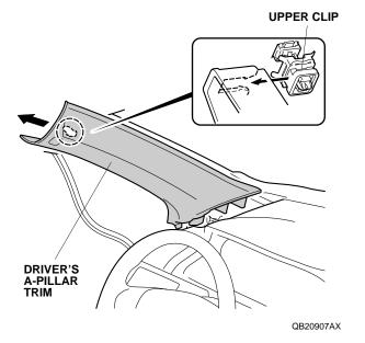
13. Remove the remaining upper clip from the driver's A-pillar.
