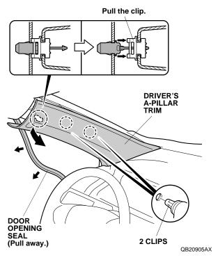
10. Pull out on the driver's A-pillar trim to release the clips.
