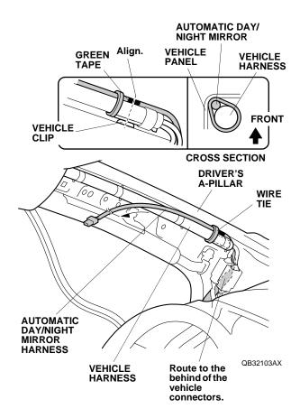
34. Route the automatic day/night mirror harness along the driver's A-pillar, and insert it under the headliner as shown. Be careful not to crease the headliner.
