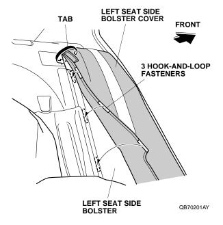
7. Insert the two tabs to the left seat side bolster.
