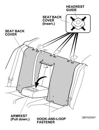
12. Insert the seat back cover between the rear seat back and the rear seat cushion, secure the four hook-and-loop fasteners to the rear seat back.
