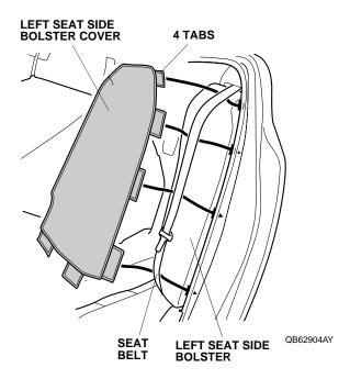
6. Insert the tab on the left seat side bolster cover to the left seat side bolster. Secure the three hook-and-loop fasteners to the left seat side bolster.
