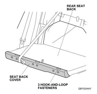
11. Insert the seat back cover under the headrest guides. Pull down the armrest, secure the hook-and-loop fastener to the rear seat back.
