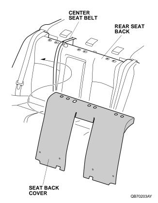
Secure the three hook-and-loop fasteners to the rear seat back. Raise the rear seat back and lock it to its original position.
