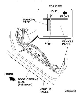
9. Attach a piece of masking tape to the vehicle panel in the location shown.
