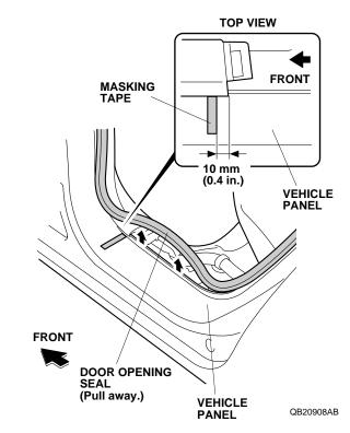
19. Attach a piece of masking tape to the vehicle panel in the location shown.
