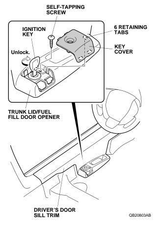
Remove one self-tapping screw from the trunk lid/ 3. fuel fill door opener cover.
