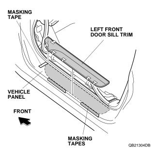
15. While applying light pressure against the left front door sill trim, carefully remove the adhesive backings.
