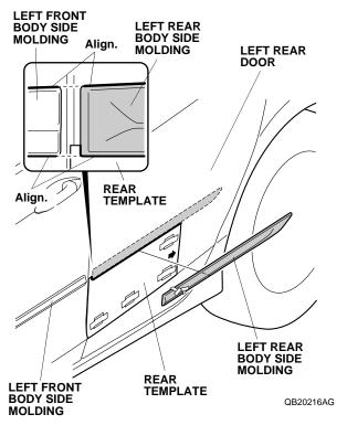
14. Make sure the edges of the left front body side molding and the left rear body side molding are aligned.
