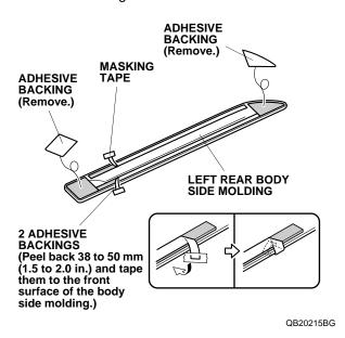
13. Align the left rear body side molding with the rear template, and attach it to the left rear door as shown.
