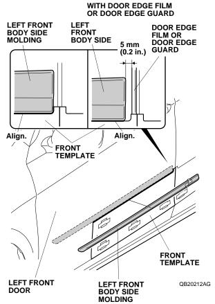
9. While applying light pressure against the left front body side molding, carefully remove the taped adhesive backings. Remove about 50 to 100 mm (2.0 to 4.0 in.) at a time.
