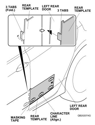
4. Insert the folded tabs of the rear template into the opening between the rear door and the B-pillar. Align the template with the character line, and tape the template to the door with strips of masking tape.
