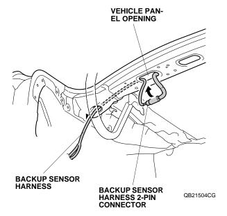
Secure the backup sensor harness to the vehicle harness with one wire tie.
