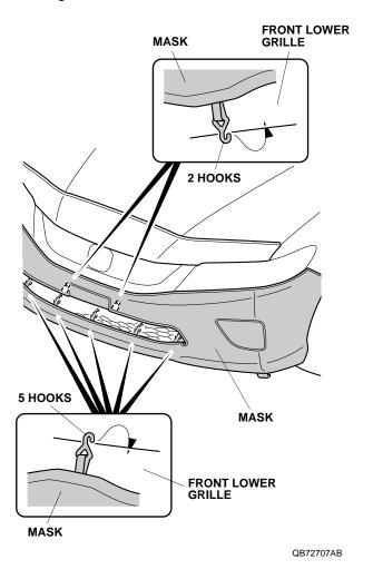
11. Attach one hook to the bottom edge of the front bumper. Repeat on the right side.
