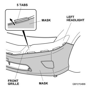
8. Pull the mask back toward the fenderwell, smooth out any wrinkles, and then snap the mask onto the snap-screw. Repeat on the right side.
