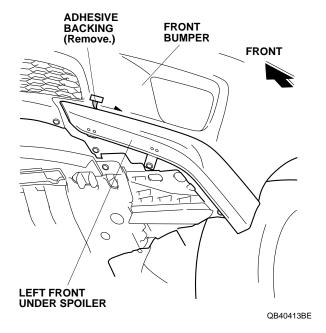
15. Using you hand, firmly press the left front under spoiler against the front bumper for 30 second.
