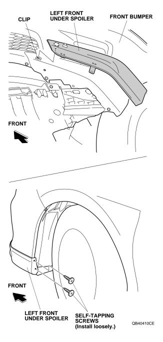
12. Secure the front portion of the left front under spoiler to the front bumper with one washer and one bumper clip supplied.
