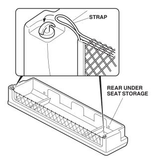
6. Position the rear under seat storage on the carpet, and align the holes in the rear under seat storage with the holes in the brackets. Secure the seat storage with the two knob bolts.
