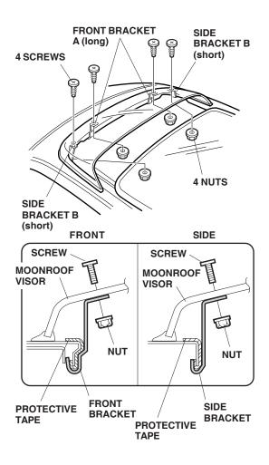
8. While holding the visor in place, install the brackets A and B with four screws and four nuts, with the end of each bracket hooked to the lip of the moonroof opening over the protective tape.
