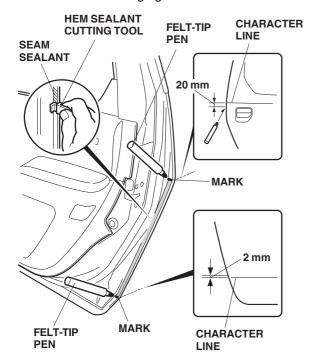
9. Position the hem sealant cutting tool against the door edge, and trim the seam sealant from mark to mark.
