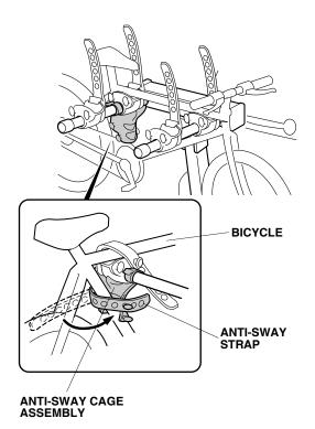
5. Using the strap provided, secure the bicycle wheels. Secure the strap buckle as shown.
