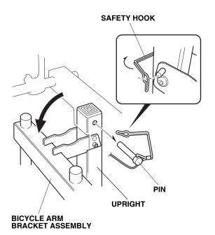
2. Reinstall the pin and safety hook as shown.
