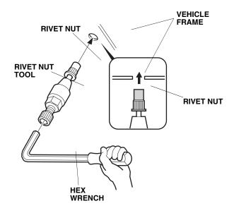
Holding the rivet nut tool with the hex wrench, turn the 27 mm wrench clockwise and install the rivet nut on the vehicle frame.
