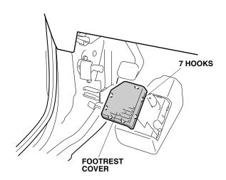
6. Remove the footrest (two flange nuts).
