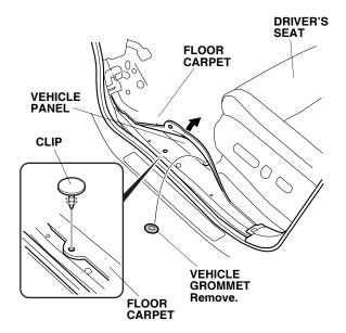
18. Remove the vehicle grommet from the floor.
