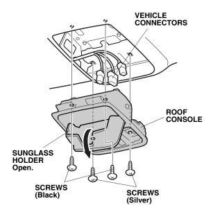
5. Remove the roof console (two black screws, two silver screws, and unplug the vehicle connectors).
