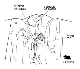
25. Continue routing the buzzer harness down along the vehicle harness, and secure it to the vehicle harness with three wire ties.
