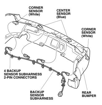
59. Secure the three backup sensor subharness clips to the three sensor clips as shown.
