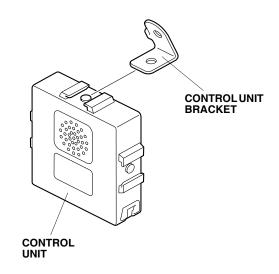
22. Secure the control unit bracket to the vehicle panel with one flange bolt and one flange nut as shown.
