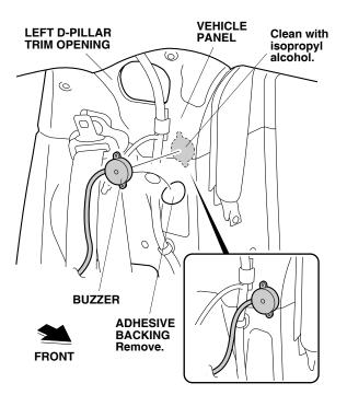
24. Route the buzzer harness along the vehicle harness, and secure it to the vehicle harness with one wire tie.
