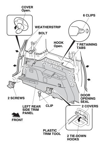
14. Pull away the weatherstrip and door opening seal at the front and rear of the left rear side trim panel. Remove the left rear side trim panel. 15. Using a rubber mallet wrapped with a shop towel, gently tap the left D-pillar trim at the area shown to release the clip.
