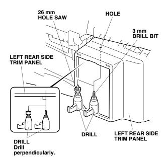
47. Install the switch into the 26 mm hole in the left rear side trim panel.NOTE: Make sure the switch is installed in the correct direction.
