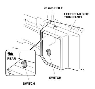
48. Using isopropyl alcohol on a shop towel, clean the switch bracket where the cushion tape will attach. Attach the remaining piece of cushion tape (from step 27.) to the switch bracket as shown.
