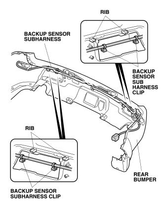
61. Secure the clip on the backup sensor subharness to the hole on the rear bumper as shown.
