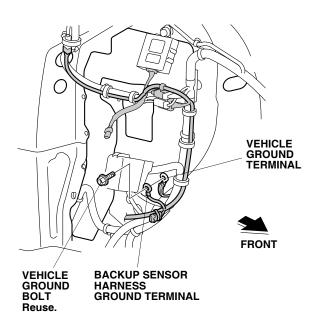
38. Route the backup sensor harness along the vehicle harness, and secure it to the vehicle harness with three wire ties.
