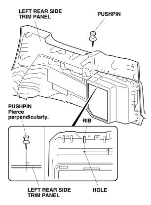
46. While wearing an eye protection, drill a 3 mm hole at the pierced mark using a 3 mm drill bit. Enlarge the 3 mm hole to 26 mm using a 26 mm hole saw. NOTE: Make sure to drill perpendicularly to the left rear side trim panel.
