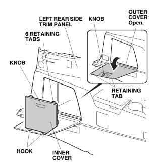
44. Pull the knob, and remove the inner cover from the left rear side trim panel (six retaining tabs and two hooks).
