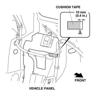
28. Using isopropyl alcohol on a shop towel, clean the vehicle panel where the cushion tape will attach. Attach the cushion tape to the vehicle panel in the area shown.
