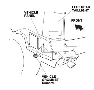
40. Route the backup sensor harness through the vehicle grommet hole, and install the backup sensor harness grommet to the vehicle panel. Make sure to install the grommet in the correct orientation. Do not pull on the backup sensor harness when installing the grommet.
