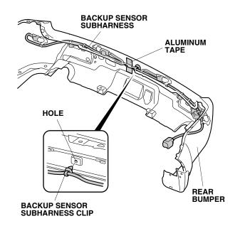
62. Using isopropyl alcohol on a shop towel, clean the rear bumper where the aluminum tape will attach. Secure the backup sensor subharness to the rear bumper with one aluminum tape.
