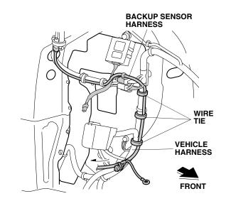
37. Remove the vehicle ground bolt from the vehicle ground terminal. Secure the backup sensor harness ground terminal to the vehicle ground terminal with the vehicle ground bolt just removed.
