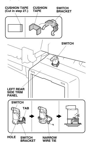
49. Secure the switch bracket to the switch using the narrow wire tie.
