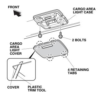
5. Remove the two bolts from the cargo area light case.
