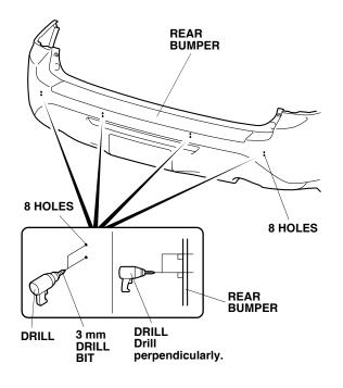
54. While wearing eye protection, enlarge the two *lower 3 mm outer* holes to 24 mm using a 24 mm hole saw.
