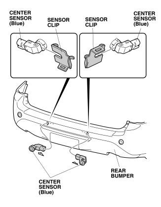
58. Plug the four backup sensor subharness 2-pin connectors into the four sensors.
