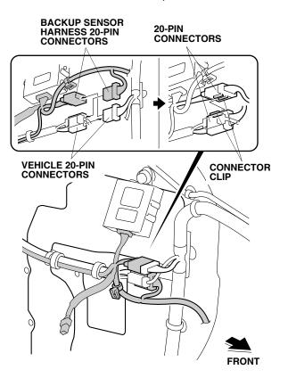
34. Attach the 20-pin connectors together using the connector clip.
