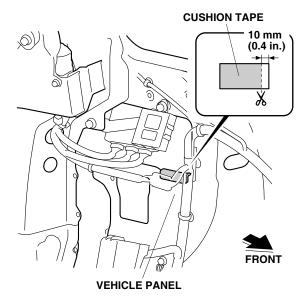
31. Using isopropyl alcohol on a shop towel, clean the vehicle panel where the cushion tape will attach. Attach the cushion tape to the vehicle panel in the area shown.
