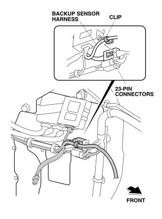
39. Route the backup sensor harness along the vehicle harness, and secure it to the vehicle harness with three wire ties.
