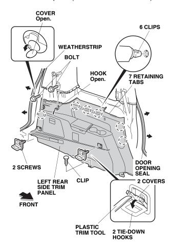
14. Pull away the weatherstrip and door opening seal at the front and rear of the left rear side trim panel. Remove the left rear side trim panel.
