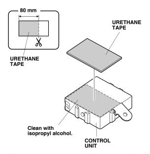
24. Using scissors, cut one urethane tape at the measurement shown. Attach the cut urethane tape to the control unit in the area shown.
