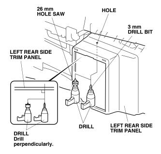
50. Install the switch into the 26 mm hole in the left rear side trim panel.
