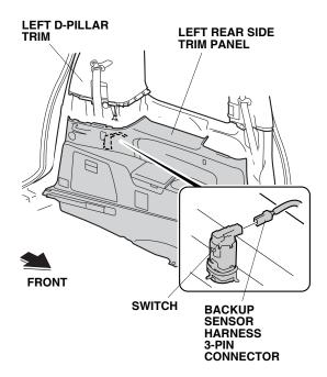
54. Bring the left rear side trim panel into position, plug the backup sensor harness 3-pin connector into the switch, and reinstall the left rear side trim panel.
