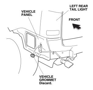
43. Route the backup sensor harness through the vehicle grommet hole, and install the backup sensor harness grommet to the vehicle panel. Make sure to install the grommet in the correct orientation. Do not pull on the backup sensor harness when installing the grommet.
