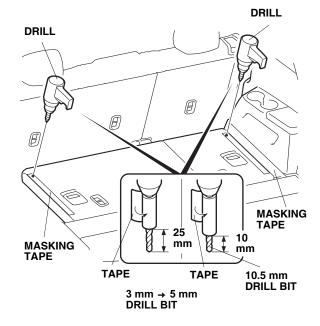
7. Drill at the marked location with a 10.5 mm drill bit. To drill through the hard board only, wrap tape around the drill bit 10 mm from the tip as shown. 8. While wearing eye protection, drill the two rear marked locations with a 3 mm drill bit and then with a 5 mm drill bit. Drill through the hard board and the sheet metal. To prevent damage to the seat, wrap tape around the drill bit 25 mm from the tip as shown.
