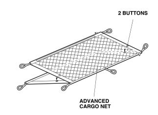
22. Attach five loops on the advanced cargo net to two anchors A (Large), two anchors B (Small) and the hook on the third row seat back board.
