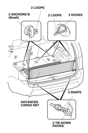
29. Attach the two snaps on the advanced cargo net to two tie-down hooks.
