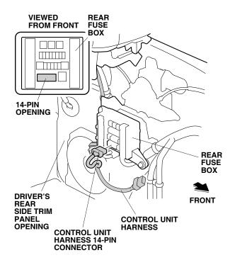
21. Install the control unit onto the control unit bracket.
