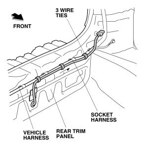
14. Plug the control unit harness 4-pin connector to the socket harness 4-pin connector.
