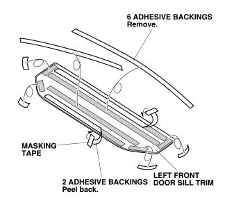
8. Remove the remaining adhesive backings.
