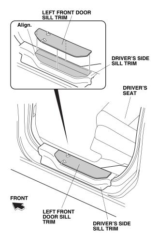
10. While applying light pressure against the left front door sill trim, carefully remove the two adhesive backings.
