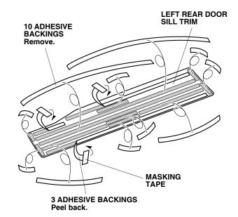
19. Remove the remaining adhesive backings.
