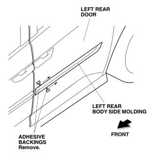
14. Using a rubber roller, apply pressure against the left rear body side molding and roll from one end to the other.
