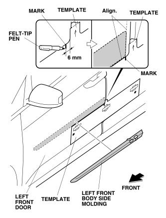
7. Align the left front body side molding with the mark on the template, and attach it to the left front door as shown.
