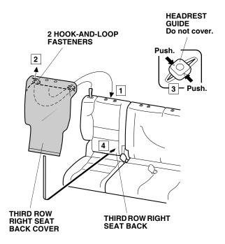
Fold down the third row right seat. Secure the third row right seat back cover to the third row right seat back with one hook-and-loop fastener. Return the third row right seat to the upright postion.
