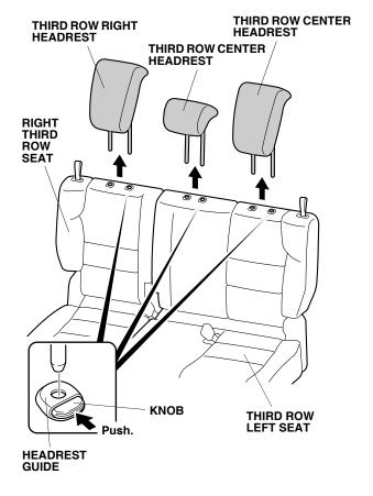
Push the knob and remove the headrests from the third row seats.  Install the two third row headrest covers and third row center headrest cover to the three headrests as shown.
