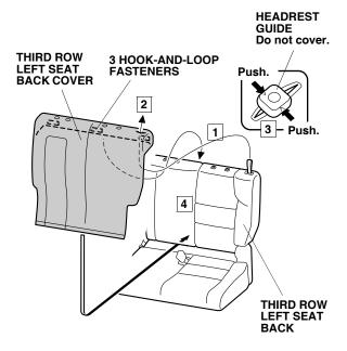
Fold down the third row left seat. Secure the third row left seat back cover to the third row left seat back with one hook-and-loop fastener. Return the third row left seat to the upright position.
