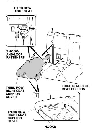
11. Secure the third row right seat cushion cover to the third row right seat cushion with the two hook-and-loop fasteners.
