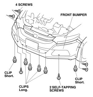
Release four retaining tabs on each side of the front bumper.
