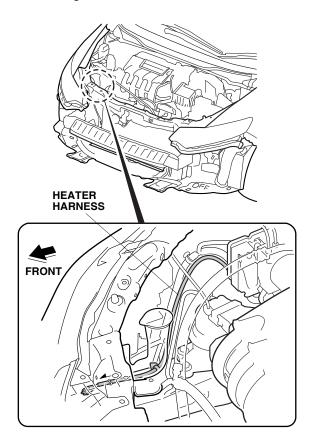
17. Secure the heater harness to the vehicle frame with one wire tie with clip (point D).
