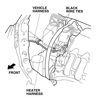
19. Secure the heater harness to the vehicle harness with three black wire ties.
