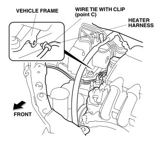
16. Route the heater harness along the vehicle harness and through the front bulkhead.
