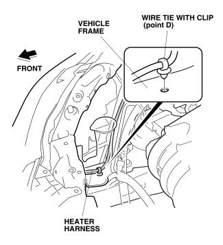
18. Secure the heater harness to the vehicle harness with two black wire ties.
