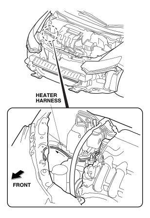
15. Secure the heater harness to the vehicle frame with one wire tie with clip (point C).
