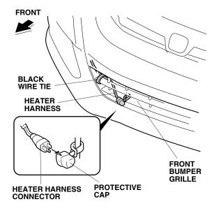
28. Secure the heater harness to the front bumper grille with one black wire tie.
