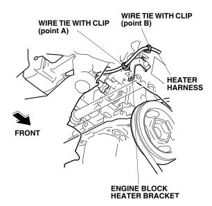
14. Route the heater harness through the engine compartment.
