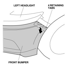
Release four retaining tabs on each side of the front bumper.
