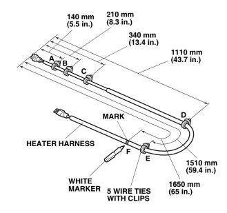
12. Plug the connector end of the heater harness into the engine block heater.
