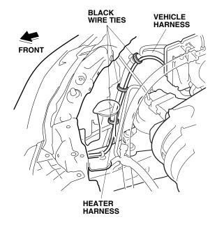
20. Route the heater harness under the frame, and secure it with one wire tie with clip (point E).
