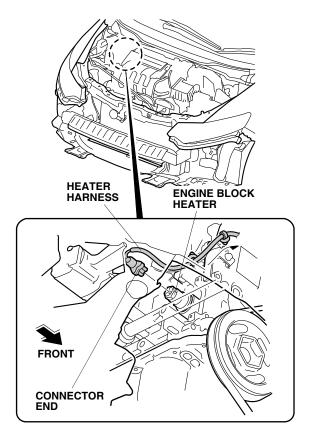
13. Route the heater harness, and secure the two wire ties with clips (points A and B) to the bracket.
