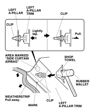
10. To release the clip, use a rubber mallet wrapped with a shop towel to lightly tap the left A-pillar trim in line with the triangular mark.
