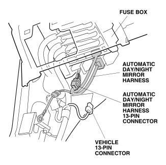
Remove and discard the upper bolt from the hood opener, and install the supplied ground bolt with the automatic day/night mirror harness ground terminal attached.
