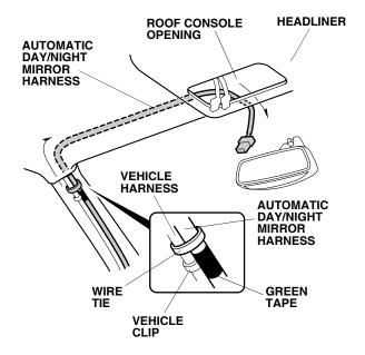
22. Secure the automatic day/night mirror harness to the vehicle harness with one wire tie at the green tape.
