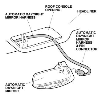
24. Route the automatic day/night mirror harness through the groove in the harness cover. Secure the harness cover to the stay, and slide the end of the harness cover under the headliner.
