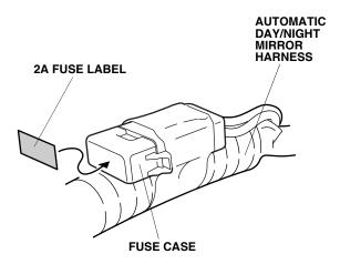
Use electrical tape to attach a piece of steel wire to the black connector on the automatic day/night mirror harness.
