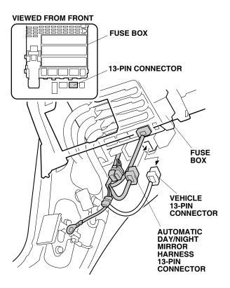
29. Plug the vehicle 13-pin connector into the automatic day/night mirror harness 13-pin connector.
