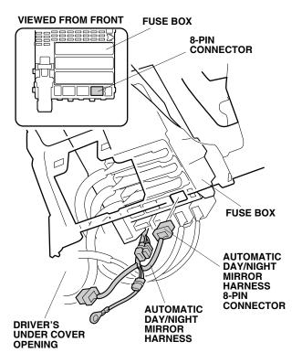
If the fog light connector is already plugged into the fuse box 8-pin connector, remove the dummy connector from the automatic day/night mirror harness.
