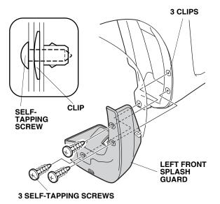
6. Check that the left front splash guard fits the contour of the vehicle.
