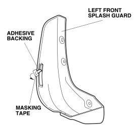
5. Loosely install the left front splash guard on the left front inner fender using three self-tapping screws.
