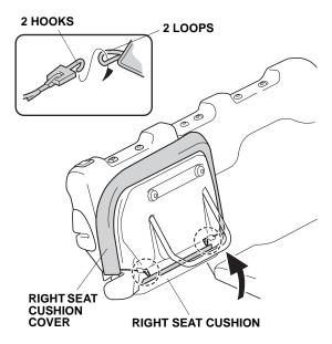
16. Lower the right seat cushion. Reinstall two seat belt buckles into the loops.
