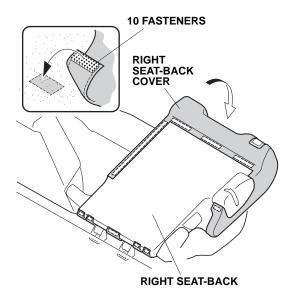
12. Lift the right seat-back. Tuck the right seat-back cover under each headrest guide as shown.
