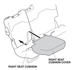
15. Lift up the right seat cushion. Secure the right seat cushion cover to the right seat cushion with two hooks and two loops.
