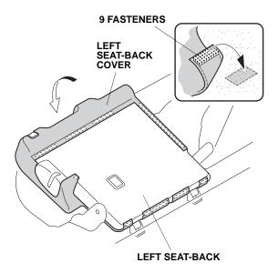
5. Lift the left seat-back. Tuck the left seat-back cover under each headrest guide as shown.
