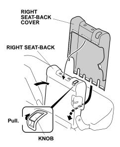
11. Fold the right seat-back fully forward. Pull the seat-back cover tight, and secure it to the right seat-back with ten hook-and-loop fasteners.
