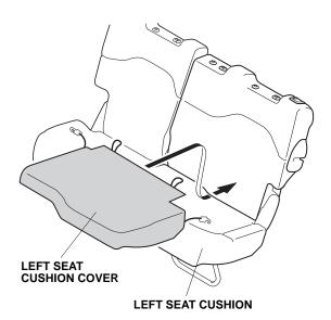
8. Lift up the left seat cushion. Secure the left seat cushion cover to the left seat cushion with two hooks and two loops.
