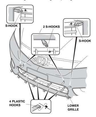
16. Route the elastic cord through the eight loops on the bottom of the mask. Attach two S-hooks and a plastic hook to the bottom of the bumper on each side.
