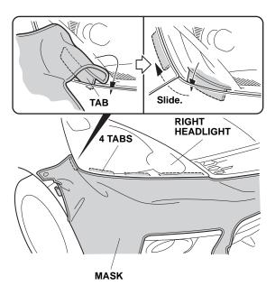
12. Pull the mask smooth, and secure the snap on the mask to the snap-screw. Attach the fourth plastic hook to the fenderwell.
