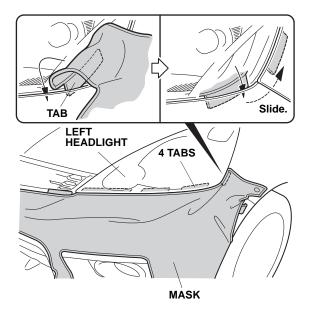
10. Insert four tabs between the front grille and the bumper.
