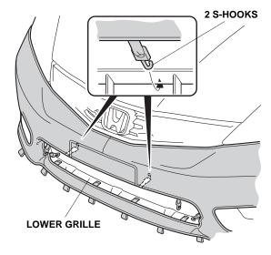
15. Attach four S-hooks to the upper edge of the lower grille opening. Attach four plastic hooks to the bottom edge of the lower grille opening.
