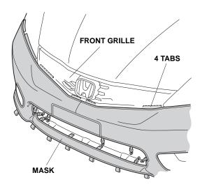
11. Insert four tabs between the headlight and the bumper.
