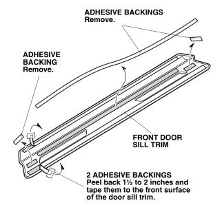
4. Using an alcohol swab, clean the surface where the front door sill trim will be installed.
