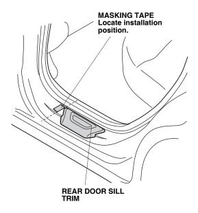
10. Peel back 1½ to 2 inches of adhesive backing from the two outer adhesive strips, and tape the ends to the front surface of the rear door sill trim. Remove the remaining three pieces of adhesive backing from the trim.
