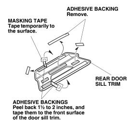
11. Using an alcohol swab, clean the surface where the rear door sill trim will be installed.
