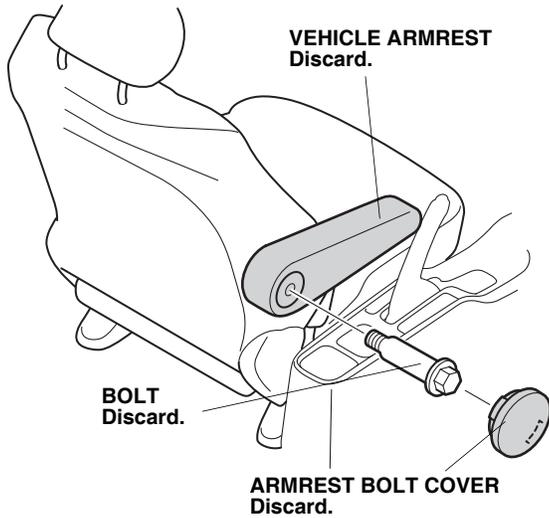
2. Remove the bolt to remove the armrest. Set the armrest aside, it will not be reused.
