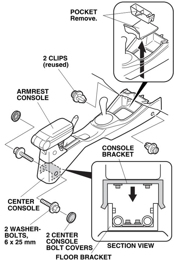
16. Carefully reinstall the center console using the two clips removed in step 7 and two 6 x 25 mm washer-bolts from the kit.
