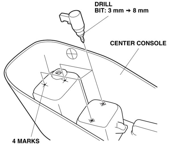
12. While wearing eye protection, drill the two pierced marks on the sides of the center console to 20 mm. First drill with a 3 mm drill bit, and finish with a 20 mm hole saw. Remove any burrs from the edges of the holes with a file.
