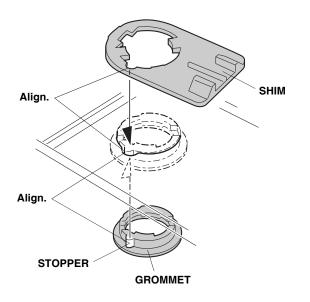
42. Attach the ambient light to the shim, and turn the ambient light clockwise to lock it in place.
