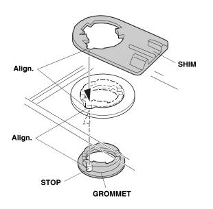
31. Attach the ambient light to the shim, and turn the ambient light clockwise to lock it in place.
