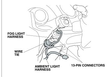
11. Using one wire tie, secure the ambient light harness to the square hole in the vehicle frame (If another accessory harness is installed, secure the ambient light harness to the other accessory harness).
