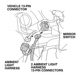
9. With accessory fog lights: Unplug the vehicle 13-pin connector from the fog light harness, and plug it into the ambient light harness 13-pin connector. Plug the other ambient light harness 13-pin connector into the fog light harness 13-pin connector.
