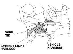
With Fog Lights: Secure the two 13-pin connectors to the fog light harness using one wire tie for each connector.
