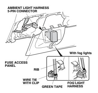
48. Using one wire tie with clip, secure the ambient light harness to the rib of the fuse access panel (If accessory fog lights are installed, secure the ambient light harness to the fog light harness).
