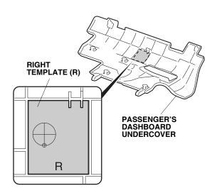
36. Using a pushpin, pierce the center of the two scribe marks on the right template (R).
