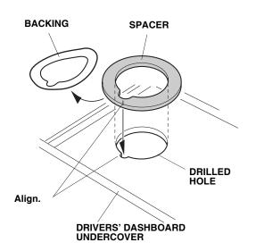
30. Align one shim and one grommet over the drilled hole as shown.
