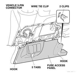
5. Remove the passenger's dashboard undercover (three clips and two tabs).
