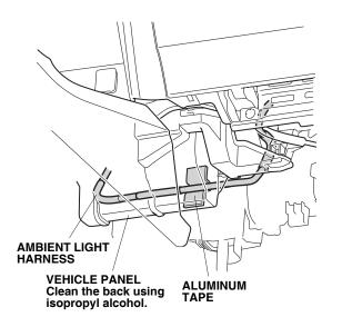
18. Using the aluminum tape, secure the ambient light harness to the back of the vehicle panel.
