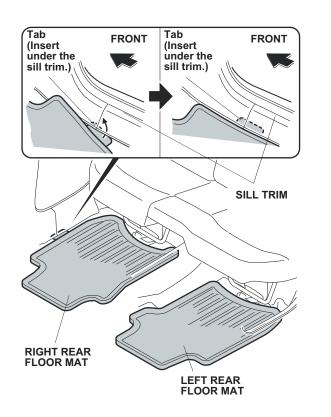
4. Install the right and left rear floor mats. Insert the tab from each floor mat under the sill trim.
