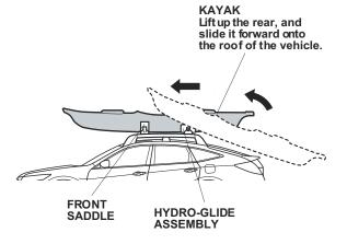
4. Adjust the distance of the saddles and hydro-glide assemblies to the same width as the kayak, then secure the saddles and the hydro-glide assemblies by tightening the knobs you installed in steps 1 and 2.
