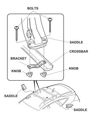
Position the two hydro-glide assemblies on the rear crossbar. Loosely install the hydro-glide assemblies with one bracket, two bolts, and two knobs for each assembly. The distance between the two assemblies should be the same width as the kayak.
