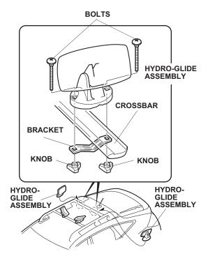
3. Rest the front of the kayak on the hydro-glide assemblies. Standing behind or alongside the kayak, lift up the rear portion of the kayak and push it forward, sliding on the hydro-glide assemblies and saddles. Make sure the kayak reaches the front saddles before you lower it.
