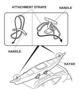
12. Attach one ratchet hook to the front attachment strap, and one ratchet hook to the rear attachment strap. Attach the front hook to the front bumper beam or tow hook. Attach the rear hook to the rear bumper beam or the trailer hitch. Secure the kayak to the vehicle by pulling the rope through the ratchet hooks.
