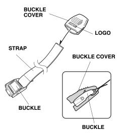
Route the strap under the front crossbar, and around the kayak as shown. Slide the buckle cover away from the buckle, route the strap through the buckle, and tighten the strap. Slide the buckle cover back over the buckle.
