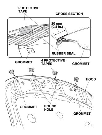
5. Remove the adhesive backings from the protective tapes and attach four protective tapes around the front of the hood under the rubber seal. Use the two grommets and the two round holes as references. Wrap approx. 20 mm (0.8 in.) of the protective tape around the lip of the hood at each of the four locations.
