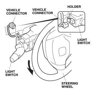
23. Remove two self-tapping screws from the light switch. While pushing the retaining tab, slide the light switch, and remove it from the steering column. Do not pull on the lever when removing the case. Do not damage the tab hole in the steering column.
