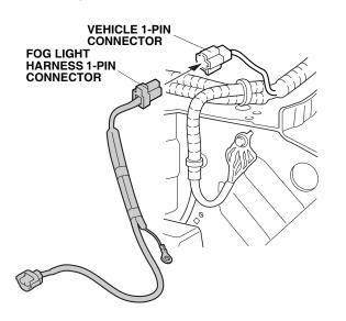
10. Secure the fog light harness ground terminal to the vehicle frame with the ground bolt supplied.
