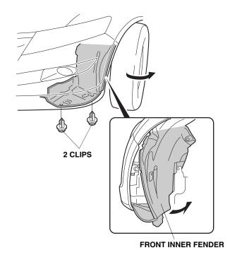
2. Insert your hand inside of the front inner fender pulled back in step 1. Unplug the fog light connector from the fog light, and remove the bulb by turning it counterclockwise.
