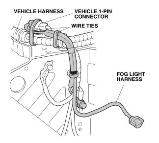
18. With the help of an assistant, bring the front bumper close to the vehicle, and plug in the fog light harness 2-pin connectors. Reinstall the front bumper.
