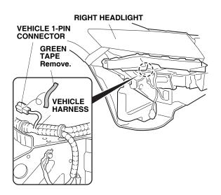
14. Plug the fog light harness 1-pin connector into the vehicle 1-pin connector.
