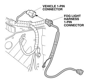
15. Locate and remove the vehicle ground bolt. Secure the fog light harness ground terminal and vehicle ground terminal to the vehicle frame with the vehicle ground bolt just removed.
