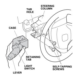
24. Holding the case in your hand, install the new lighting switch to the steering column. Install the two self-tapping screws. Do not push on the lever when installing the case. Push on the case and set the retaining tab in to the tab hole.
