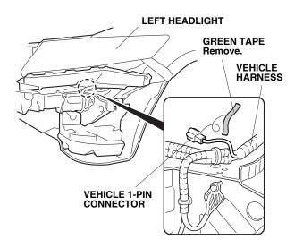
9. Plug the fog light harness 1-pin connector into the vehicle 1-pin connector.
