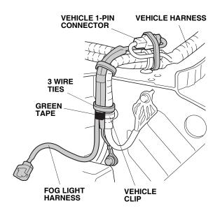
12. Secure the fog light harness and vehicle 1-pin connector to the vehicle harness with two wire ties.
