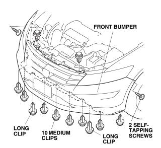
• With the help of an assistant, remove the front bumper. Place the front bumper on a blanket to prevent damage.
