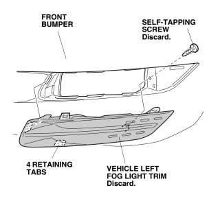
5. Install the new left fog light trim to the front bumper with four retaining tabs.
