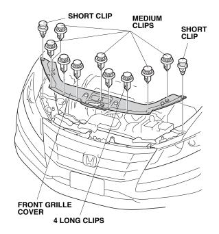
• Remove 2 self-tapping screws, 2 long clips, and 10 medium clips.
