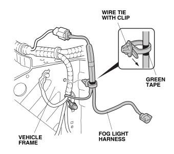
17. Secure the fog light harness and vehicle 1-pin connector to the vehicle harness with two wire ties.
