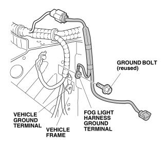
16. Secure one wire tie with clip to the fog light harness at the green tape. Secure the wire tie with clip to the hole in the vehicle frame.
