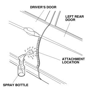
Open the driver's door again. Peel back about 50 mm (2 in.) of adhesive backing from the left front door edge film. Align the V-notch in the door edge film with the end of the character line on the upper part of the door.
