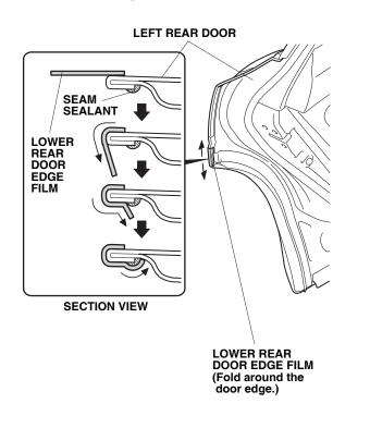
24. Using a lint-free shop towel, wipe the 3M protective tape application solution from the lower rear door edge film. Allow the lower rear door edge film to dry thoroughly.
