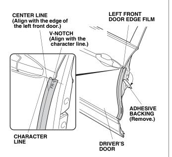
4. Continue to remove the adhesive backing while you align the center line of the door edge film with the edge of the door.
