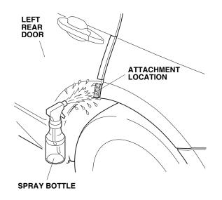
Open the left rear door. Peel back about 25 mm (1 in.) of adhesive backing from the lower rear door edge film. Align the V-notch with the top of the arch in the rear door.
