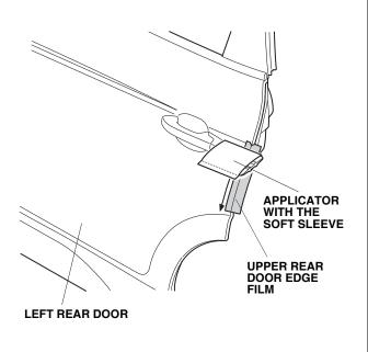
14. When you are satisfied that the upper door film is firmly attached to the edge of the door, slowly remove the outer protective film.
