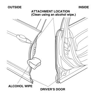
2. Close the driver's door. Using a spray bottle with 3M protective tape application solution, spray the area where the left front door edge film will attach.
