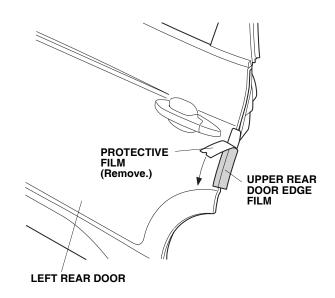
15. Starting from the middle of the upper door edge film and working outward, fold the upper rear door edge film around the door edge using your fingers. Move your fingers in one direction. Attach the film over the seam sealant. Do not trim or damage the seam sealant.
