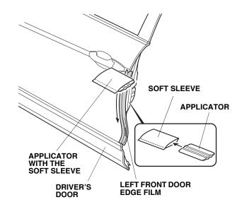
6. When you are satisfied that the door film is firmly attached to the edge of the door, slowly remove the outer protective film.
