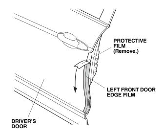
7. Starting from the middle of the door edge film and working outward, fold the left front door edge film around the edge of the driver's door using your fingers. Move your fingers in one direction. Attach the film over the seam sealant. Do not trim or damage the seam sealant.
