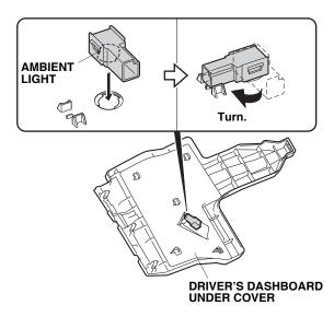
21. Plug the ambient light harness 2-pin connector into the ambient light, and reinstall the driver's dashboard under cover.
