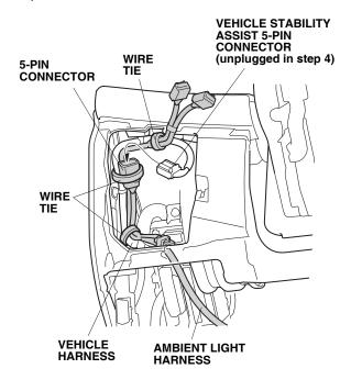
13. Using three wire ties, secure the ambient light harness to the vehicle harness.
