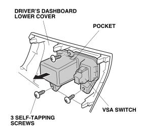
8. Remove the VSA switch (two retaining tabs).
