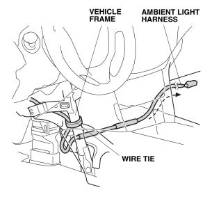
19. Continue routing the ambient light harness along the vehicle harness, and secure the ambient light harness to the vehicle harness using five wire ties.
