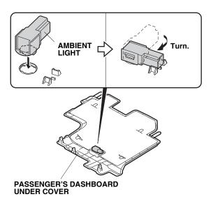
23. Plug the ambient light harness 2-pin connector into the ambient light, and reinstall the passenger's dashboard under cover.
