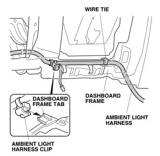
16. Using one wire tie, secure the ambient light harness to the dashboard frame.
