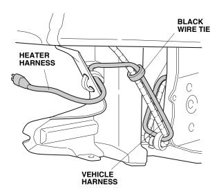
23. With the help of an assistant, route the heater harness through the grille opening in the bumper, then reinstall the front bumper.
