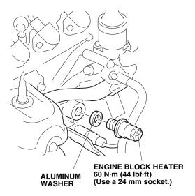
11. Plug the connector end of the heater harness into the engine block heater.
