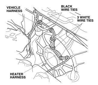
16. Route the heater harness down and under the vehicle frame as shown.
