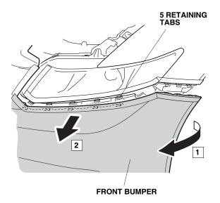
With the help of an assistant, remove the front bumper (two hex bolts and two clips). Place the front bumper on a blanket to prevent damage.
