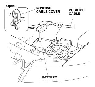
7. Remove the two nuts from the battery setting plate, then remove the battery setting plate and J-bolts. Remove the battery upper cover, the battery, and battery under cover.
