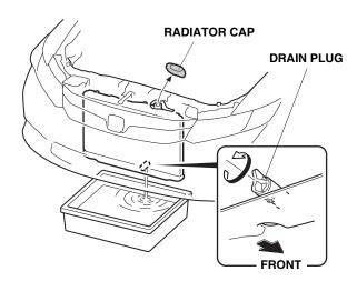
4. Drain the coolant completely, then loosely reinstall the radiator cap.
