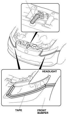
Remove the 2 self-tapping screws, 10 short clips, and 2 long clips. Note the locaion of the two long clips.
