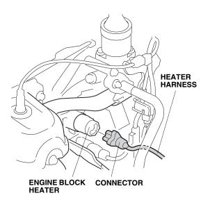
12. Secure the heater harness to the vehicle bracket with one white wire tie at the mark you made (Point A).
