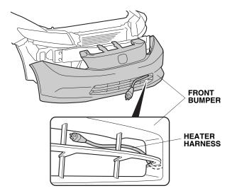
24. Route the heater harness inside the front bumper and secure it to the grille support with one black wire tie.
