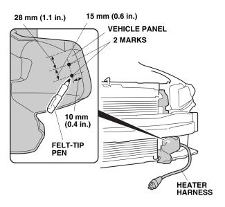
20. Using a pushpin, pierce the two marks on the vehicle panel. While wearing eye protection, drill the two pierced marks with a 3 mm drill bit, then enlarge the holes with a 5 mm drill bit. Remove any burrs.
