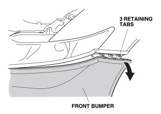
On each side, release five retaining tabs.
