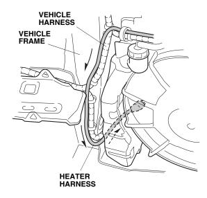
17. Using two black wire ties, secure the heater harness to the vehicle harness.
