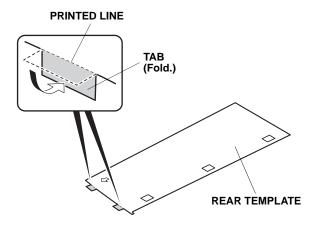
5. Position the two tabs on the rear template against the front edge of the left rear door.
