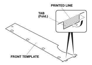
2. Position the two tabs on the front template against the rear edge of the left front door.
