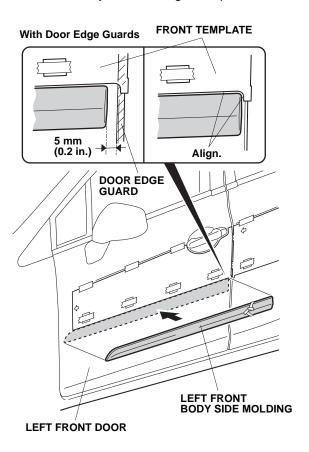
11. Press on the left front body side molding firmly with the palm of your hand while removing about 50 to 100 mm (2.0 to 3.9 in.) of the adhesive backing at a time.
