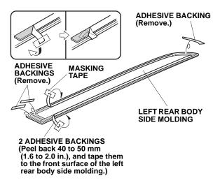
14. Align the edges of the left rear body side molding with the edges of the rear template, and attach the left rear body side molding to the left rear door.
