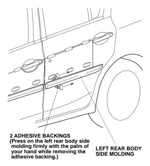
16. Using a rubber roller, apply firm pressure, especially at the ends, to set the adhesive.
