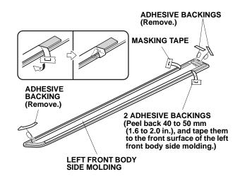
10. Align the edges of the left front body side molding with the edges of the front template, and attach the left front body side molding to the left front door. If the vehicle is equipped with door edge guards, attach the left front body side molding at the position shown.
