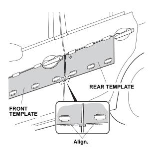
Using two alcohol wipes, clean the surfaces of both doors where the body side moldings will attach.
