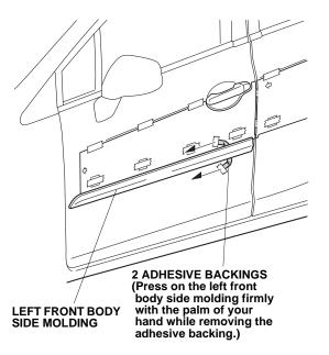
12. Using a rubber roller, apply firm pressure, especially at the ends, to set the adhesive.
