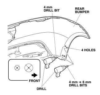
16. Enlarge the two front holes in the rear bumper with a 6 mm drill bit. Remove any burrs.
