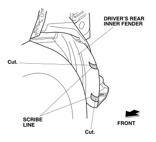
20. Using a utility knife, cut off the tab in the driver's rear inner fender as shown.
