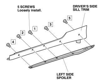
10. Tighten the middle screw loosely installed in step 9.
