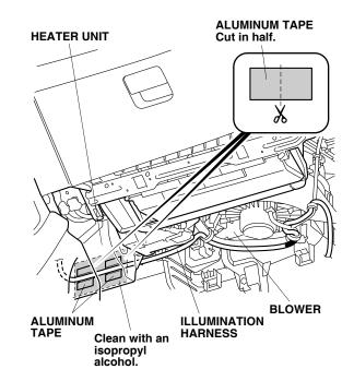
53. Using scissors, cut one aluminum tape in half. Secure the illumination harness to the back of the heater unit with two pieces of aluminum tape as shown. 54. Route the illumination harness to the passenger's kick panel opening.
