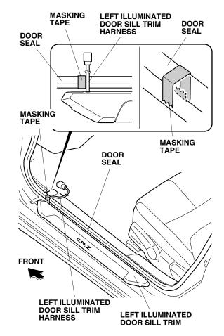
13. Route the left illuminated door sill trim harness over the door seal. Attach a piece of masking tape to the door seal to mark where the illuminated door sill trim harness crosses the door seal. 14. Pull up the door seal from the door sill trim at the masking tape.
