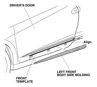
Peel back approximately 1½ to 2 inches of adhesive backing from each adhesive strip, and tape the ends to the front surface of the body side molding.
