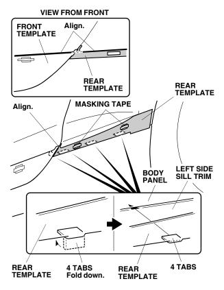
6. Align the rear template to the body panel and attach it with masking tape.
