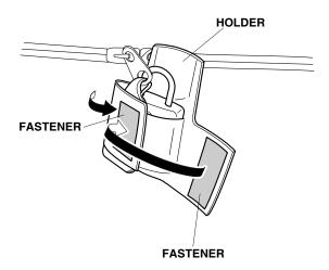
22. Secure two buckles on the cargo bag and pull the excess belt on the buckles to tighten.
