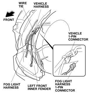
31. Secure the fog light harness to the vehicle harness with one wire tie. Do not secure the fog light harness to the SRS harness.
