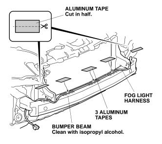
39. Cut one aluminum tape in half. Secure the fog light harness to the bumper beam with the two halves of aluminum tape.
