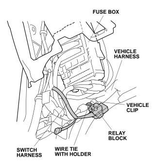
48. Plug the switch harness 1-pin connector to the vehicle 1-pin connector.
