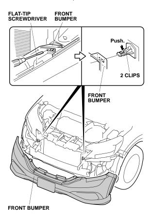
With the help of an assistant, remove the front bumper. Place the front bumper on a blanket. 24. Remove the four clips, and release the left front inner fender. Do not fully remove the left front inner fender.
