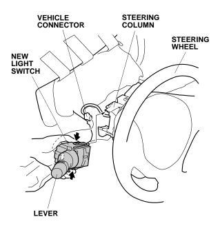
60. Plug the vehicle connector into the new light switch.
