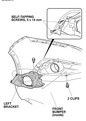
28. Install the fog light to the front bumper with two 5 x 14 mm self-tapping screws.
