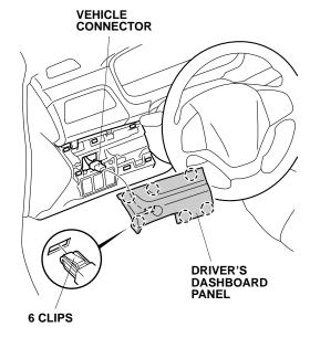
3. Remove the driver's dashboard under cover (turn the knob, one clip, and one pin).
