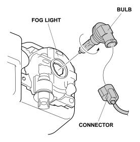
3. Remove the bulb by turning it counterclockwise.
