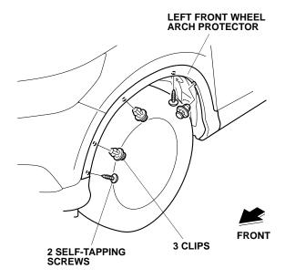
15. Remove the left front wheel arch protector (eight clips and three retaining tabs).
