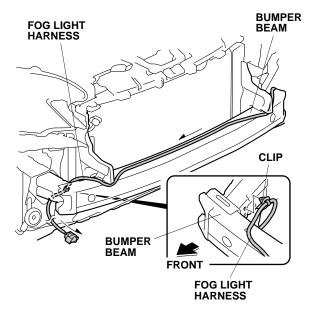
38. Using isopropyl alcohol on a shop towel, thoroughly clean the areas where the aluminum tapes will attach. Secure the fog light harness to the bumper beam with three aluminum tapes.
