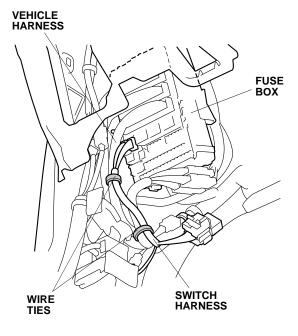
57. Unplug the vehicle connector from the light switch.
