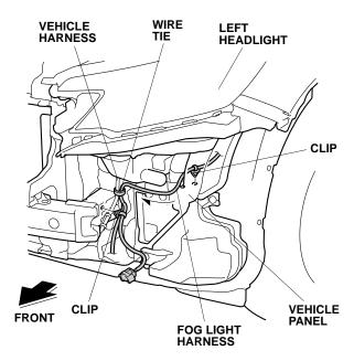
36. Secure the fog light harness to the vehicle harness with one wire tie.
