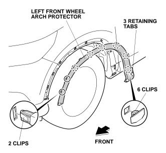
16. Repeat steps 14 and 15 to remove the front wheel arch protector from the right side of the vehicle.
