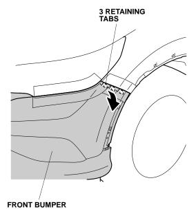
Release the four retaining tabs on each side.
