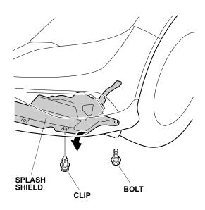
2. Insert your hand behind the splash shield. Unplug the connector from the fog light.
