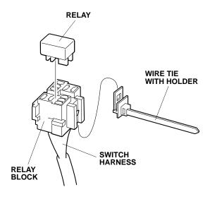
46. Install the wire tie with holder onto the switch harness relay block.
