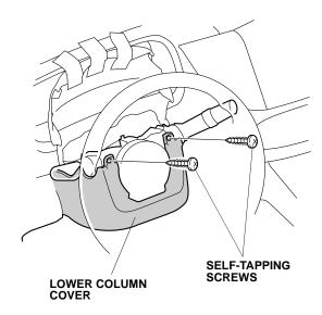
11. Remove the lower column cover (one self-tapping screw).
