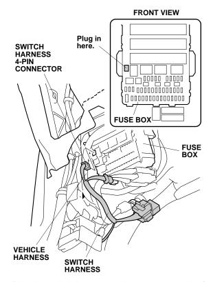
50. Plug the switch harness 4-pin connector to the fuse box. Go to step 53.
