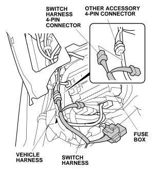
52. Plug the switch harness 4-pin connector to the other accessory's 4-pin connector.
