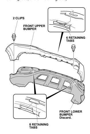
26. Install the new front lower bumper with six retaining tabs, eight retaining tabs, and two clips.
