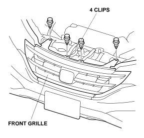
20. Using a flat-tip screwdriver, release the front grille (four clips).
