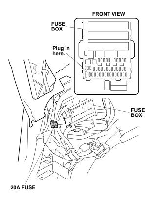
62. Using isopropyl alcohol on a shop towel, thoroughly clean the area where the fuse label will attach. Attach the fuse label to the fuse box label on the driver's dashboard under cover.
