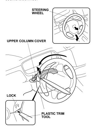
7. Using a plastic trim tool, release the lock as shown.
