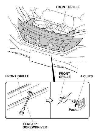
21. Using a long shank flat-tip screwdriver, release the one clip and two retaining tabs.
