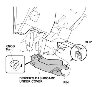
4. Remove the driver's dashboard lower cover (eight clips and unplug the vehicle connector).
