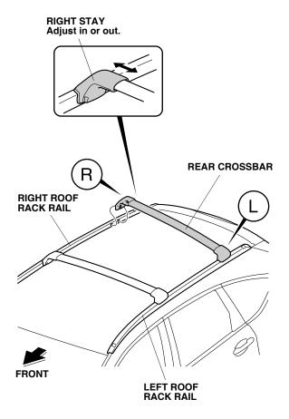
5. Secure the rear crossbar to the roof rack rails using four bolts. Torque the bolts to 10 N·m (7.3 lbf·ft).
