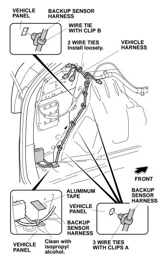
41. Route the backup sensor harness along the vehicle harness. Secure it to the vehicle panel and vehicle harness with three wire ties with clips A, one wire tie with clip B, and two loosely-installed wire ties.
