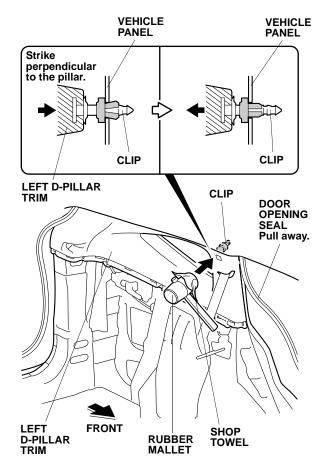
19. Using a rubber mallet wrapped with a shop towel, lightly tap the area marked "SIDE CURTAIN AIRBAG" on the left D-pillar trim to push in the clip. Make sure to tap perpendicular to the pillar.
