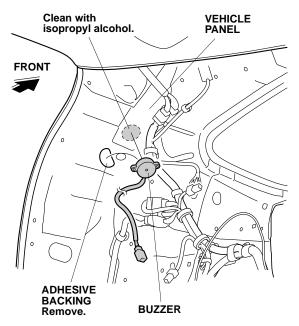
51. Remove the adhesive backing from the buzzer and attach the buzzer to the vehicle panel in the location shown.
