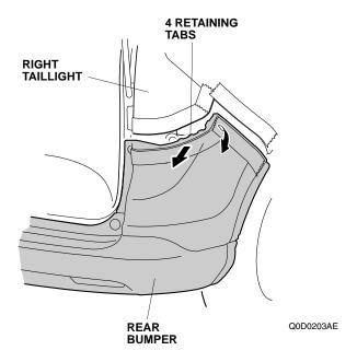
With the help of an assistant, remove the rear bumper. Place the rear bumper on a blanket.
