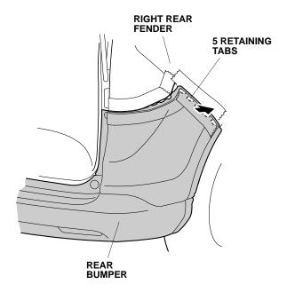
• Release four retaining tabs on each side.
