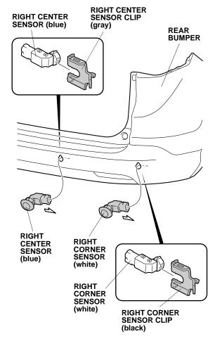
72. Secure the right corner sensor (white) and the right center sensor (blue) with the right corner sensor clip (black) and the right center sensor clip (gray) as shown.
