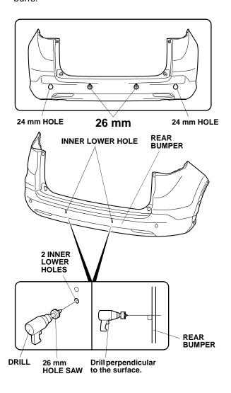
69. Insert the left corner sensor (white) and the left center sensor (blue) into the rear bumper. NOTE: The left corner sensor (white) and the left center sensor (blue) have the yellow dot.
