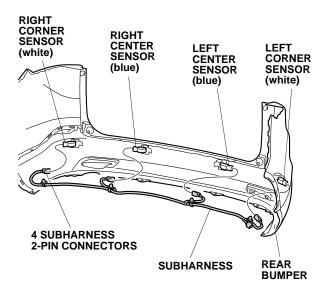
74. Secure the four backup sensor clips into the four sensor clips.
