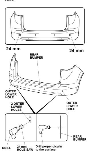
68. While wearing eye protection, enlarge the two lower inner holes with a 26 mm hole saw. Drill perpendicular to the rear bumper. Remove any burrs.
