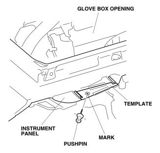
While wearing eye protection, drill a 7 mm hole through the instrument panel at the pierced mark. First drill with a 3 mm drill bit, then finish with a 7 mm drill bit. Remove any burrs.
