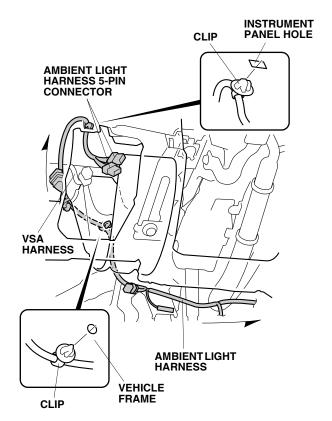
18. Secure the other ambient light harness clip to the hole in the vehicle frame.
