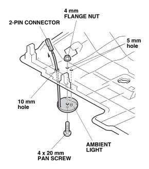
Plug the ambient light 2-pin connector to the ambient light harness 2-pin connector, and secure the 2-pin connector to the vehicle harness with one wire tie. Then, reinstall the passenger's dashboard under cover.
