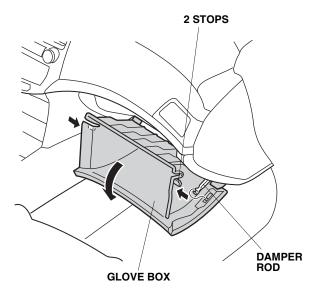
10. Remove the glove box (two screws).
