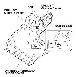
Using a utility knife, cut out the driver's dashboard under cover as shown.
