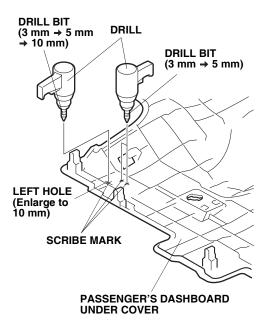
Route the ambient light 2-pin connector through the 10 mm hole, and attach the ambient light to the passenger's dashboard under cover with one 4 x 20 mm pan screw and one 4 mm flange nut through the 5 mm hole.
