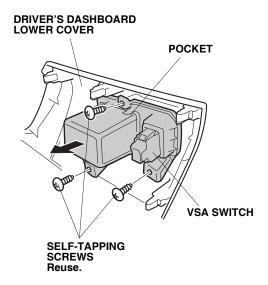
Release two retaining tabs and remove the VSA switch from the pocket. Set the pocket aside, it will not be reused.
