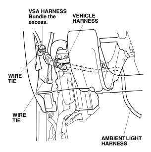
21. Secure the ambient light harness to the vehicle harness with one wire tie.
