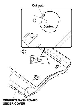
Route the ambient light 2-pin connector through the 10 mm hole, and attach the ambient light to the driver's dashboard under cover with one 4 x 20 mm pan screw and one 4 mm flange nut through the 5 mm hole.
