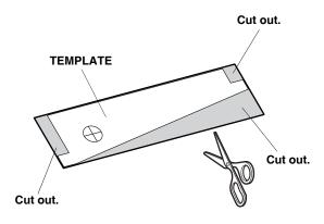
Under the glove box opening, align the template with the instrument panel.
