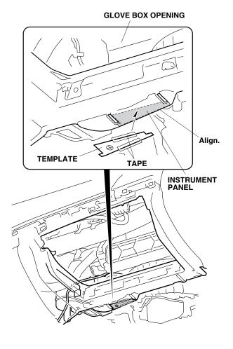
• Using a pushpin, pierce the instrument panel at the mark. Remove the template.
