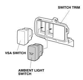
Install the switch trim to the driver's dashboard lower cover with the three self-tapping screws removed in step 11.
