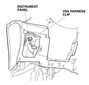
17. On the driver's side of the vehicle, route the ambient light harness 5-pin connectors up to the VSA harness. Secure the clip near the ambient light harness 5-pin connectors to the instrument panel hole where you removed the VSA harness clip.
