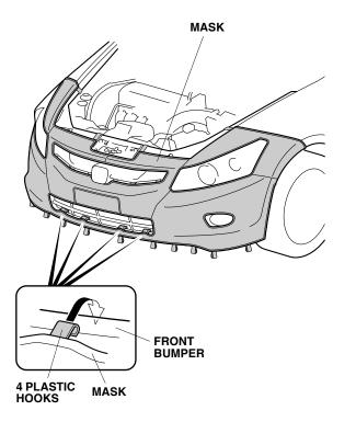
18. Route the elastic cord through the twelve loops on the bottom of the mask. Attach one hook to the hole in the inner fender. Stretch the elastic cord and attach the other hook to the inner fender hole on the other side.
