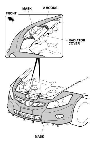
14. Attach four plastic hooks to the inside edge of the front bumper.
