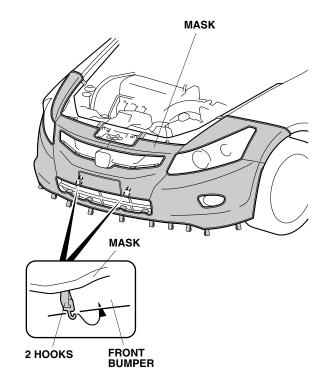
17. Attach four plastic hooks to the inside edge of the front bumper.
