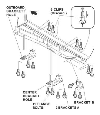
7. Install the two brackets A and one bracket B to the body using 11 flange bolts. Thread the flange bolts in about 3 to 4 threads. When installing brackets A, use the outboard bracket holes for the front bracket, and the center bracket holes for the center and rear brackets. 8. Install the side step to the brackets using 12 flange bolts and 12 flange nuts. Thread the flange bolts in about 3 to 4 threads.
