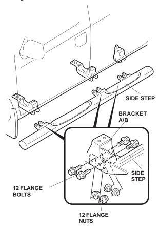
Adjust the location of the left side step so there is even clearance between the side step and body, then tighten the flange bolts you installed in step 7. Torque 10 flange bolts to 27 N·m (20 lbf·ft), and the one remaining flange bolt to 7 N·m (5 lbf·ft) as shown.
