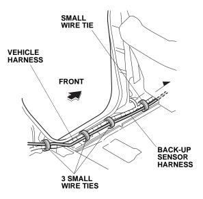
98. Route the back-up sensor harness along the vehicle harness, and secure it to the vehicle harness with three small wire ties.
