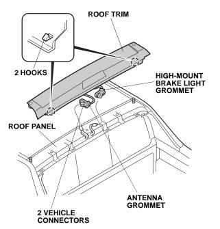
37. Remove the antenna grommet and high-mount brake light grommet from the roof panel, unplug the vehicle connectors, and remove the roof trim. 38. Remove seven vehicle grommets from the roof panel, and install six new oval grommets and one new round grommet into the roof panel as shown.
