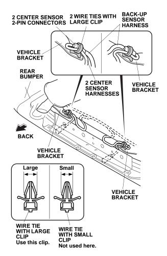
88. Inside of the vehicle, turn over the floor mat, and route the back-up sensor harness across the vehicle panel and alongside the vehicle harness.
