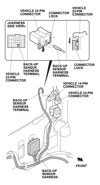
95. Push the back-up sensor harness terminal into the vehicle 23-pin connector, then reattach the connector lock. Re-plug the vehicle 23-pin and 14-pin connectors.
