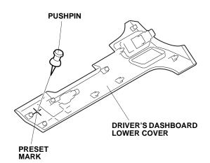
107. While wearing eye protection, drill one 26 mm hole through the marked position. First drill with a 3 mm drill bit, then finish with a 26 mm hole saw. Remove any burrs.
