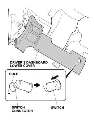
109. Plug the back-up sensor harness 3-pin connector into the switch.
