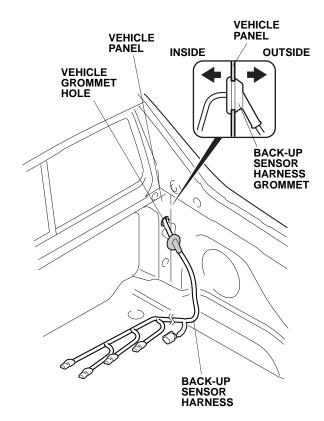
74. Install a wire tie with small clip at the green tape on the back-up sensor harness as shown. Inside the cargo area, route the back-up sensor harness along the vehicle harness, and secure the front of the back-up sensor harness to the hole on the vehicle panel with one wire tie with small clip.
