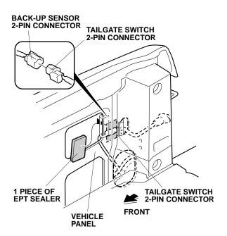
81. Using isopropyl alcohol on a shop towel, clean the area where the EPT sealer will attach. Secure the back-up sensor harness to the vehicle frame with one piece of EPT sealer.
