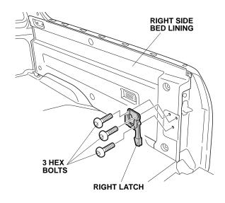
49. Remove the right side bed lining (five T-40 torx bolts, one clip, and unplug the vehicle connector).
