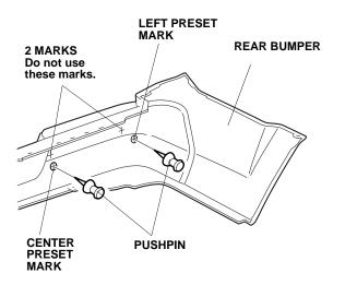
55. While wearing eye protection, drill one 20 mm hole through the outer mark, and one 26 mm hole through the inner mark on the rear bumper. First drill with a 3 mm drill bit, then finish the outer hole with a 20 mm hole saw and finish the inner hole with a 26 mm hole saw. Remove any burrs. Repeat the same procedure for the right side.
