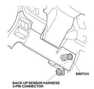
110. Using isopropyl alcohol on a shop towel, clean the area where the EPT sealer will attach. Attach the EPT sealer to the driver's console side trim in the area shown.
