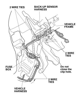
If the vehicle is equipped with the security system: Wrap one cushion tape around the back-up sensor harness, and secure it to the security system bracket with one wire tie.
