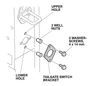
65. Install the tailgate switch bracket to the vehicle with two 4 x 14 mm washer-screws.
