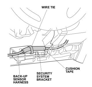
101. Route the back-up sensor harness along the vehicle harness, and secure it to the vehicle harness with three wire ties. If there is any excess, bundle it to the vehicle harness after step 105.
