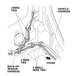
97. Route the back-up sensor harness along the vehicle harness, and secure it to the vehicle harness with four small wire ties.
