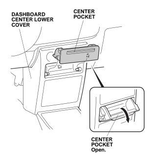
8. Remove the dashboard center lower cover (three self-tapping screws, five clips, six retaining tabs, and unplug the vehicle connectors).
