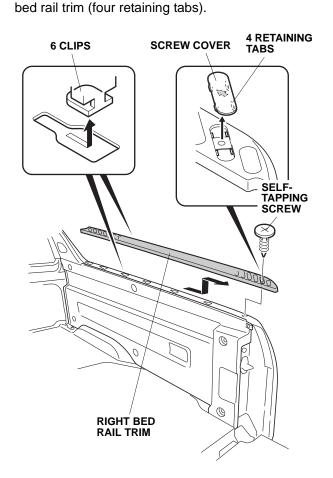
40. Remove the screw cover from the rear of the right
