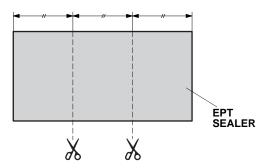
79. Using isopropyl alcohol on a shop towel, clean the areas where the EPT sealers will attach. Attach two pieces of EPT sealer to the edge of the vehicle panel as shown.
